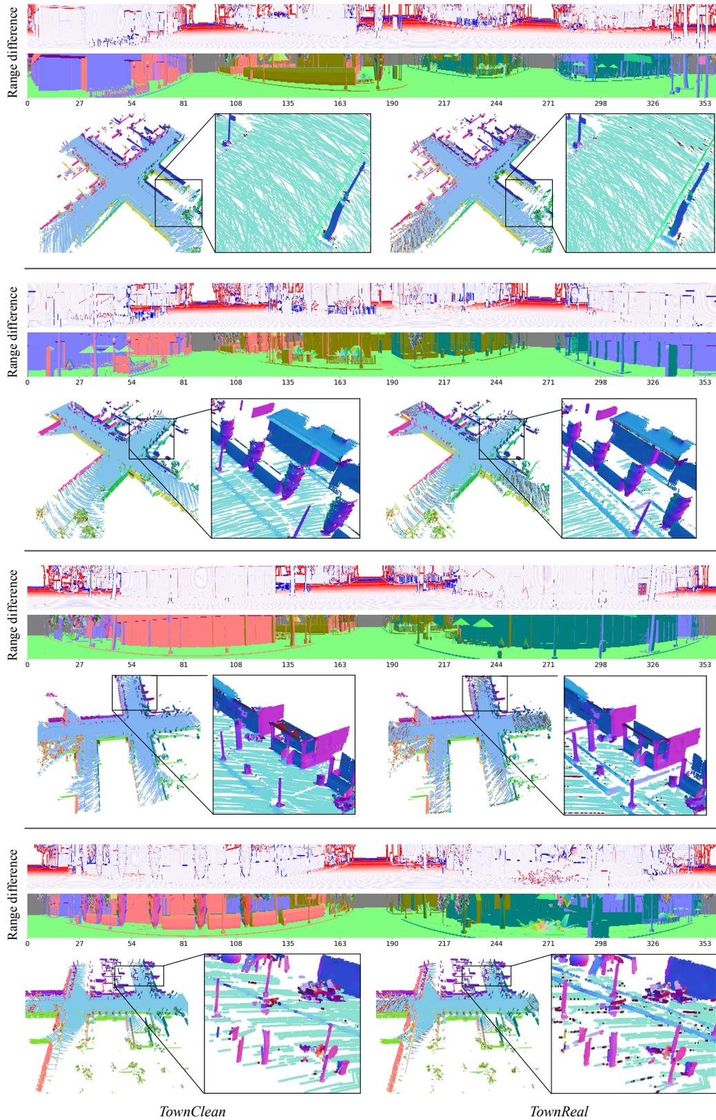
Figure 3. Visualisation of *Town* dataset. Employing a diverged beam profile in range simulation results in an overestimation of range in the high range regime (-16 █ █ 16 cm). Such range difference is also reflected on delicate structures, as evidenced by the point cloud view.
