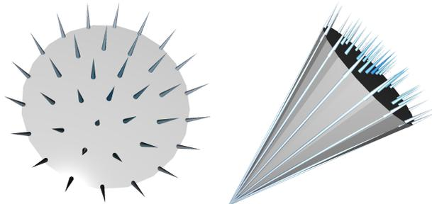
Figure 1. Example diverged beam profile approximated via 37 diverged rays.
