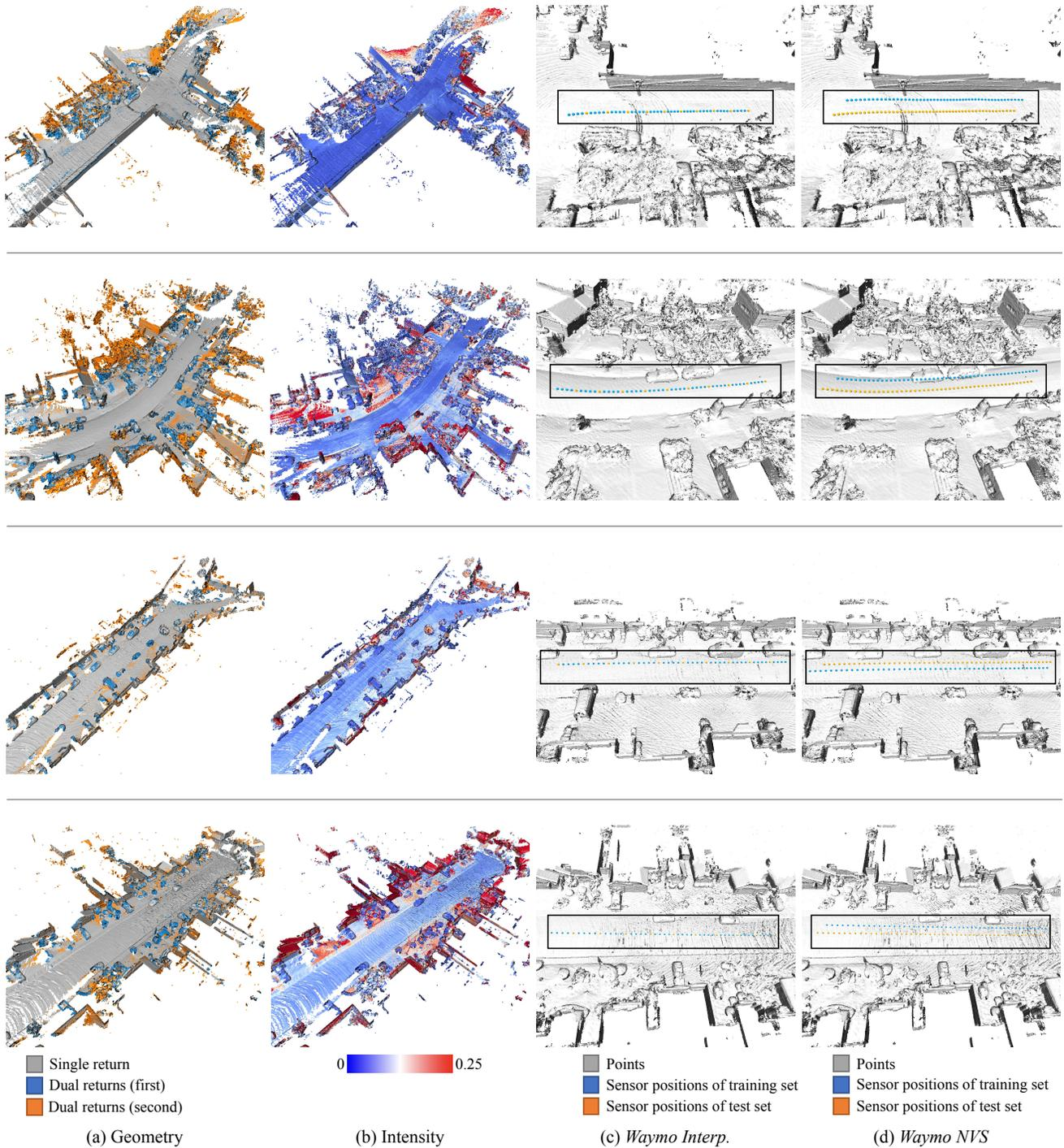
Figure 4. Visualisations of *Waymo* dataset. We accumulate all 50 frames for each scene and show their geometry, intensity profile, and sensor positions of training and test sets on *Waymo Interp.* and *Waymo NVS* datasets.
