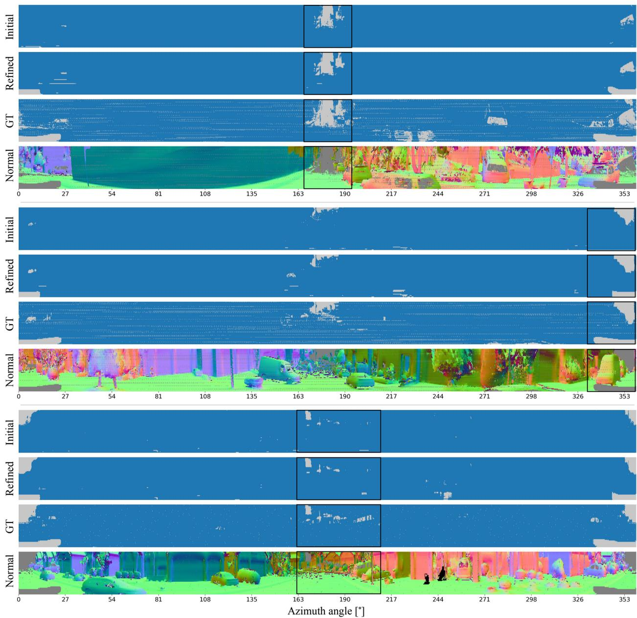
Figure 5. Ray drop segmentation on *Waymo Interp.* dataset using LiDARsim [6]. We show both the initial ray drop mask from ray-surfel query and the refined masks using learned ray-drop model.
